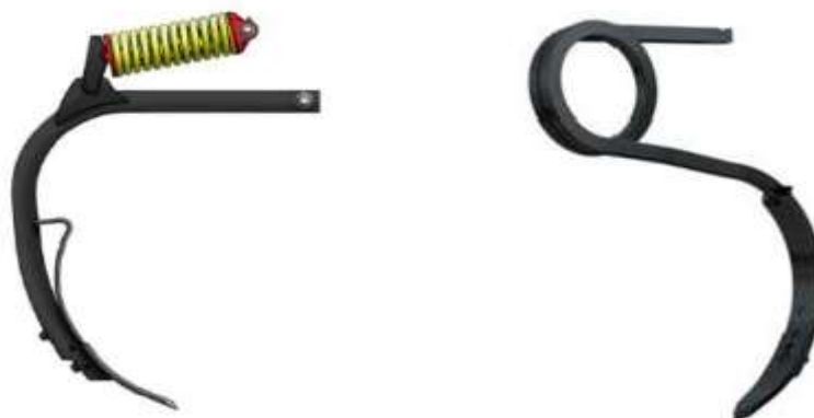
Figure 4. Elastic supports for the working bodies of cultivators
