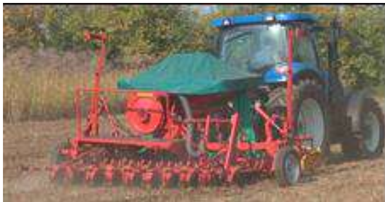
Figure 3. Technical equipment endowed with working parts for preparing the soil and sowing straw cereals
