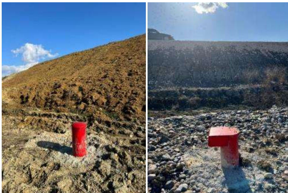
Figure 2. Photos of the piezometers that are installed in the TWTA
