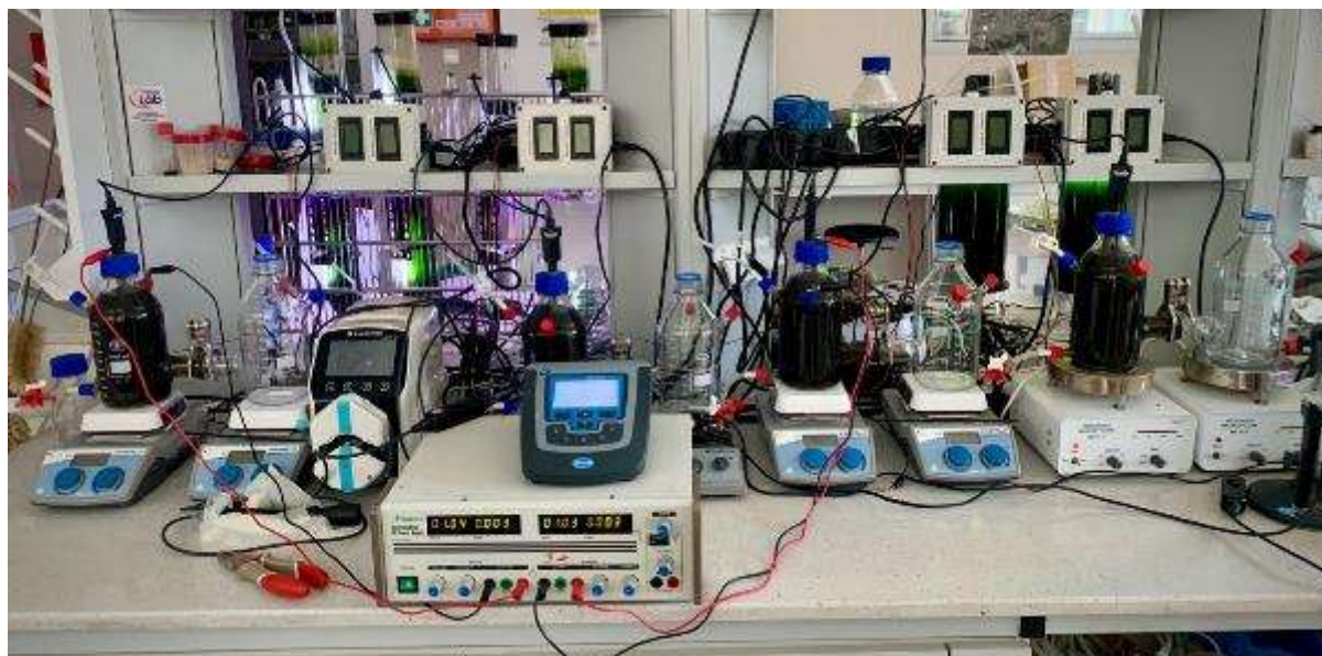
Figure 2 pMFC reactors laboratory setup with electric stimulation (R1 and R3).
