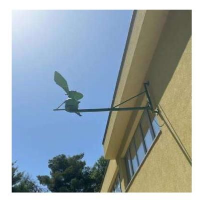
Picture 2. Burkard's volumetric pollen and spore collector
