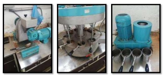
Figures 1. From left to right: crusher, malaxer and centrifuge.
