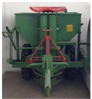
Figure 1. Image of a semi-automatic potato planter
