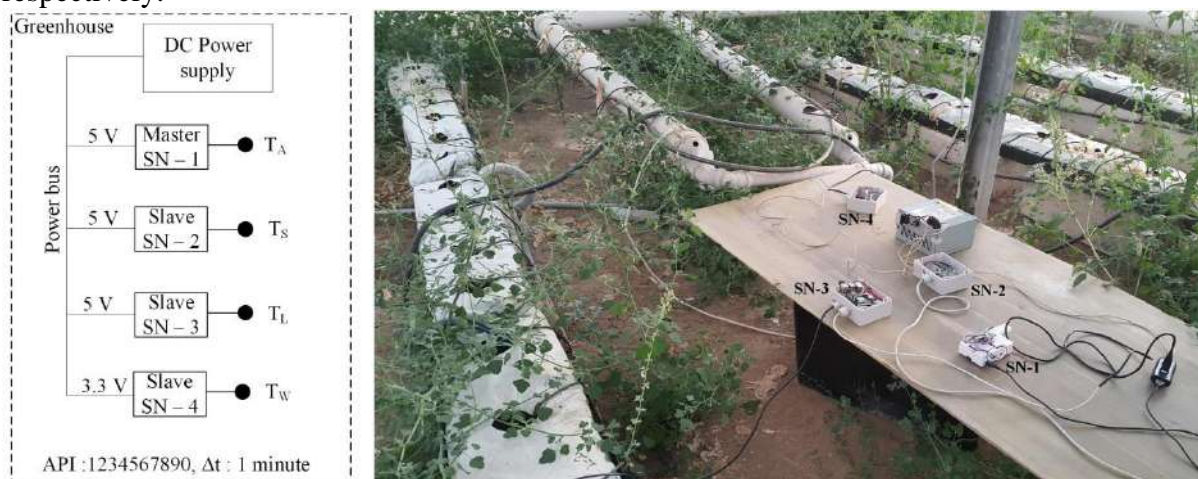
Figure 3 (a) Positions of sensor nodes in greenhouse, (b) Greenhouse experiments
