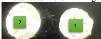
Figure 3: comparison of the clots formed from pasteurized milk using infrared radiation (1) and Classic method (2) at 72° C for 15 seconds.
