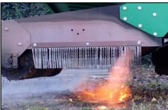
Figure 3: intensive flames under the heat chamber
