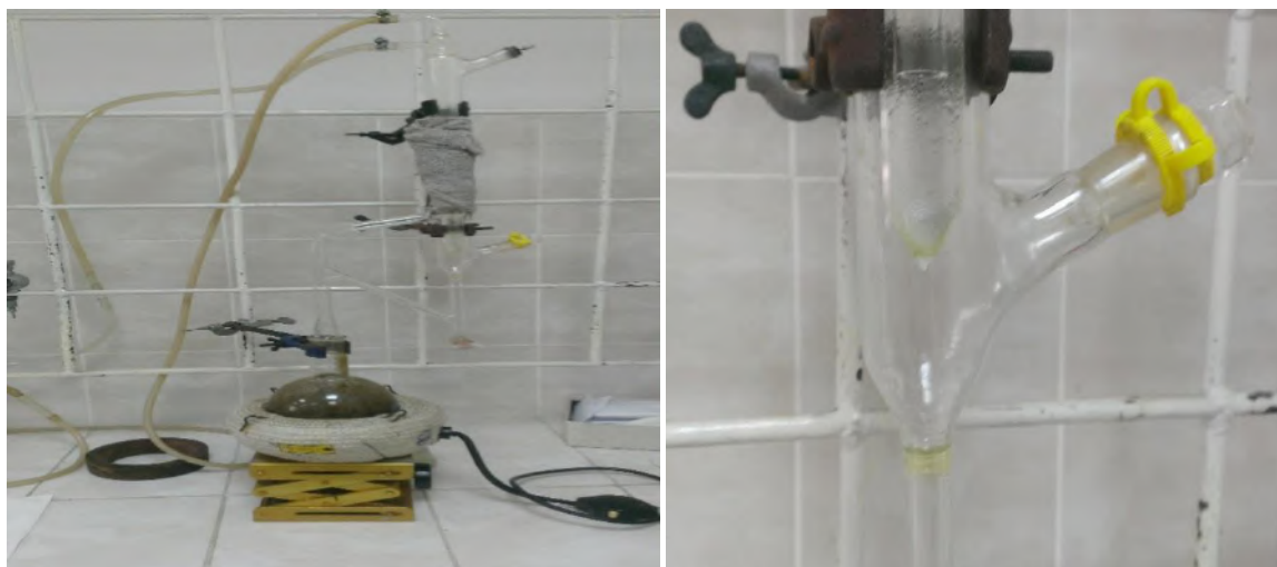
Fig. 1. Isolation of essential oil from Mentha piperita L. by hydrodistillation.
