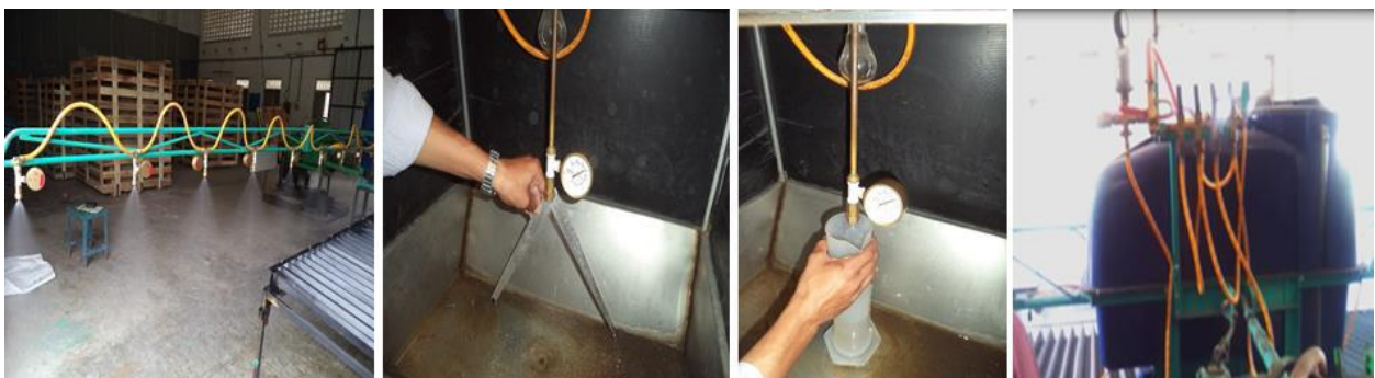
Fig.3.3. Nozzle discharge rate (Lit./Min.), Pressure (Kpa) for old and new boom design in Lab.
